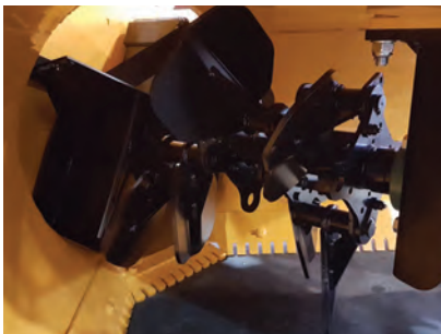
Free-swinging rotor blades
